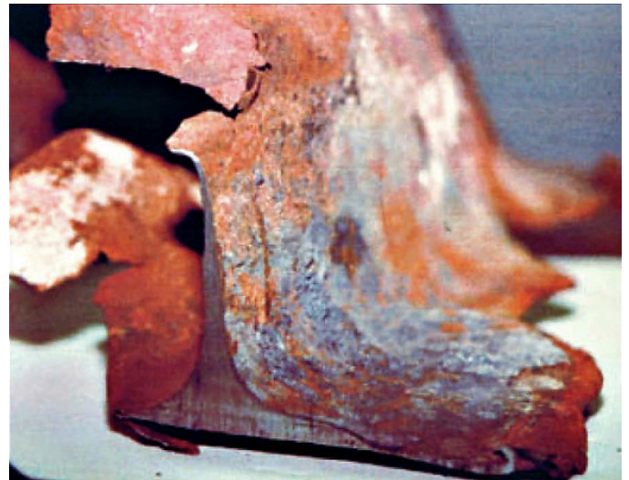
Figure 3: WTC steel sample after hot corrosion attack. FEMA, Appendix C.
