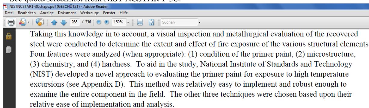
Microstructure, chemistry and hardness were only examined in a few pieces where the paint based screening process suggested a possible exposure to temperatures above 250 °C, and in sample (2) of FEMA Appendix C.
