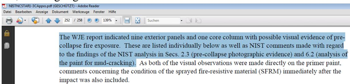
NIST's "observations" in these list are not based on the condition of the actual steel, but on the paint-cracking method. NIST notes whether a mud-cracking pattern of the paint was observed or not, and if paint was left on the piece. In addition, NIST lists the results of its fire exposure maps (which are based on videos and photos from September 11, 2001), and if the SFRM was lost or more likely not (based on the named photos and videos too). When no paint
